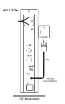
**Note:** If your TV has only 300-ohm VHF screw terminals, use a 75-ohm-to-300-ohm matching transformer to complete the connection.
